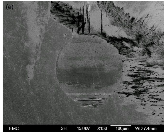
Figure 5.13: SEM images of the ball wear scars tested against MoSe 2 /DLC-W coating in PAO4-lubricated sliding at different loads: (a) 10 N, (b) 20 N, (c) 30 N, (d) 40 N, and (e) 50 N. Note that the images are at different magnifications.
