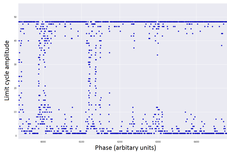
FIGURE K.3: Data shown is the expanded version of the data in the red box shown in figure K.2. The size of the dataset makes the regions of chaotic motion difficult to see without zooming in as such. Transitional behaviour between bimodal duffing oscillator and chaotic behaviour (vertical line sections) for limited values of driving phase.
