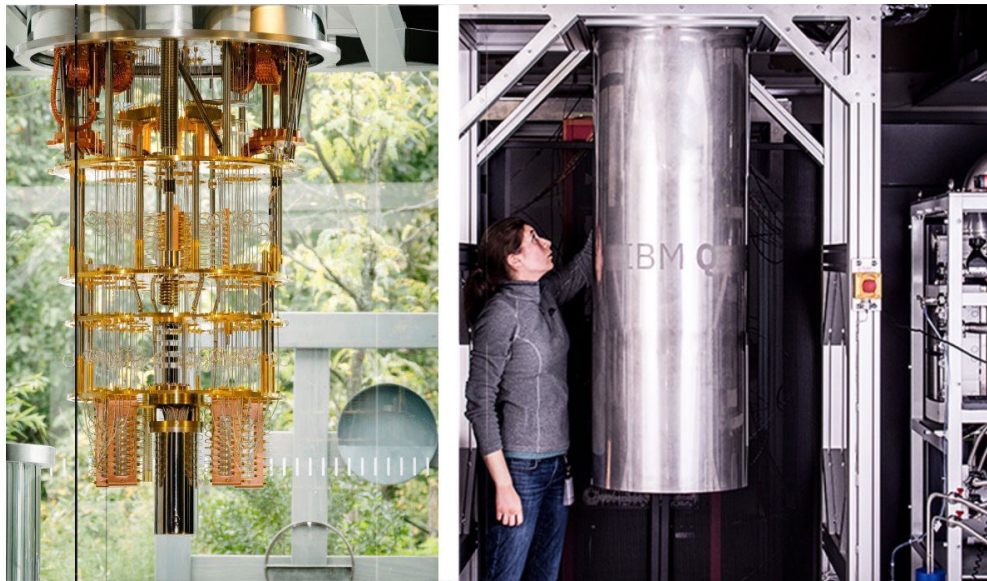
Figure 4.6: An illustration of IBM’s quantum computer that utilises superconducting circuits. ©IBM. Source: (Hui 2019).
