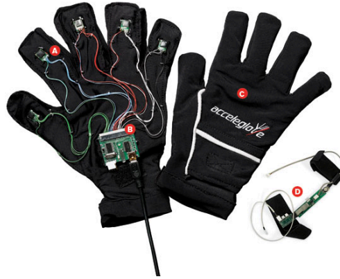
Figure 2.12: AcceleGlove - a programmable open-source data glove (Grifantini, 2009).
