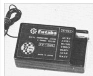
1980 - 6 channel 27 MHz Futaba FP5LK RC transmitter and receiver
