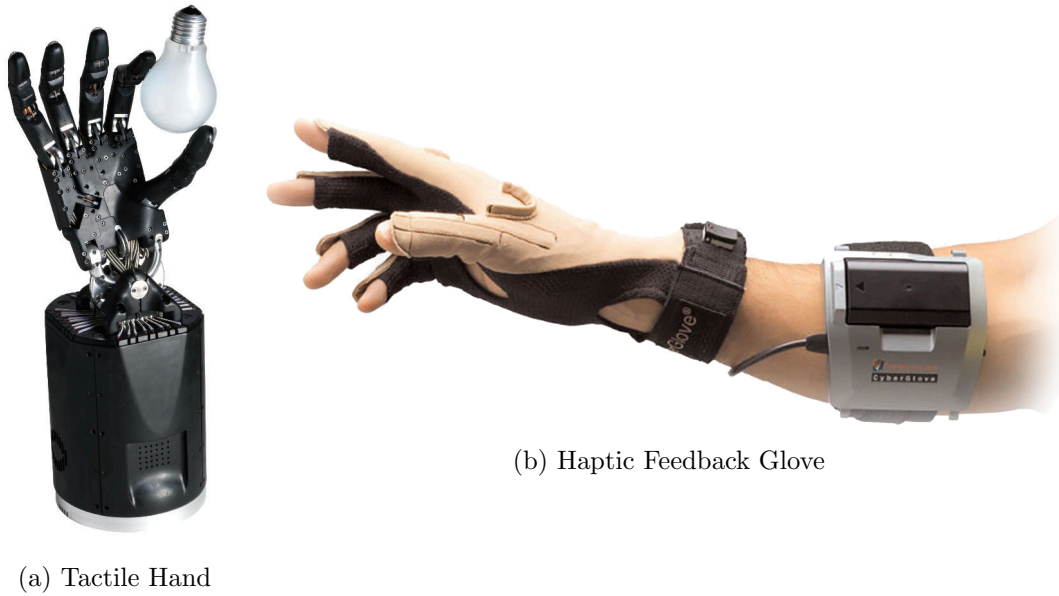
Figure 2.11: Tactile sensitive robot hand ( Shadow Robot, 2013 ) integrate-able with the haptic feedback gloves ( Cyber Glove, 2009 ).
