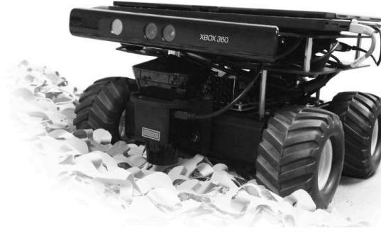
Figure 2.26: JRMBot Platform with the Kinect and a laptop computer installed (Harris and Barber, 2014).
