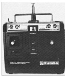
1980 - 6 channel 27 MHz Futaba FP5LK RC transmitter and receiver
