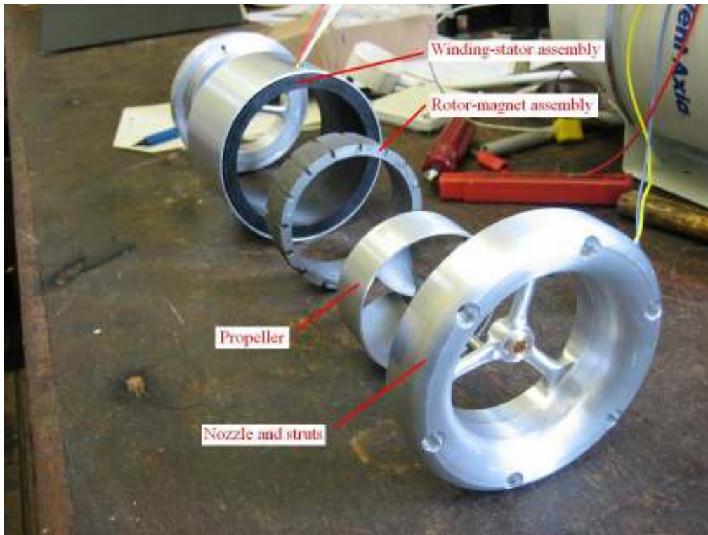
Figure 38: Thruster parts expanded
