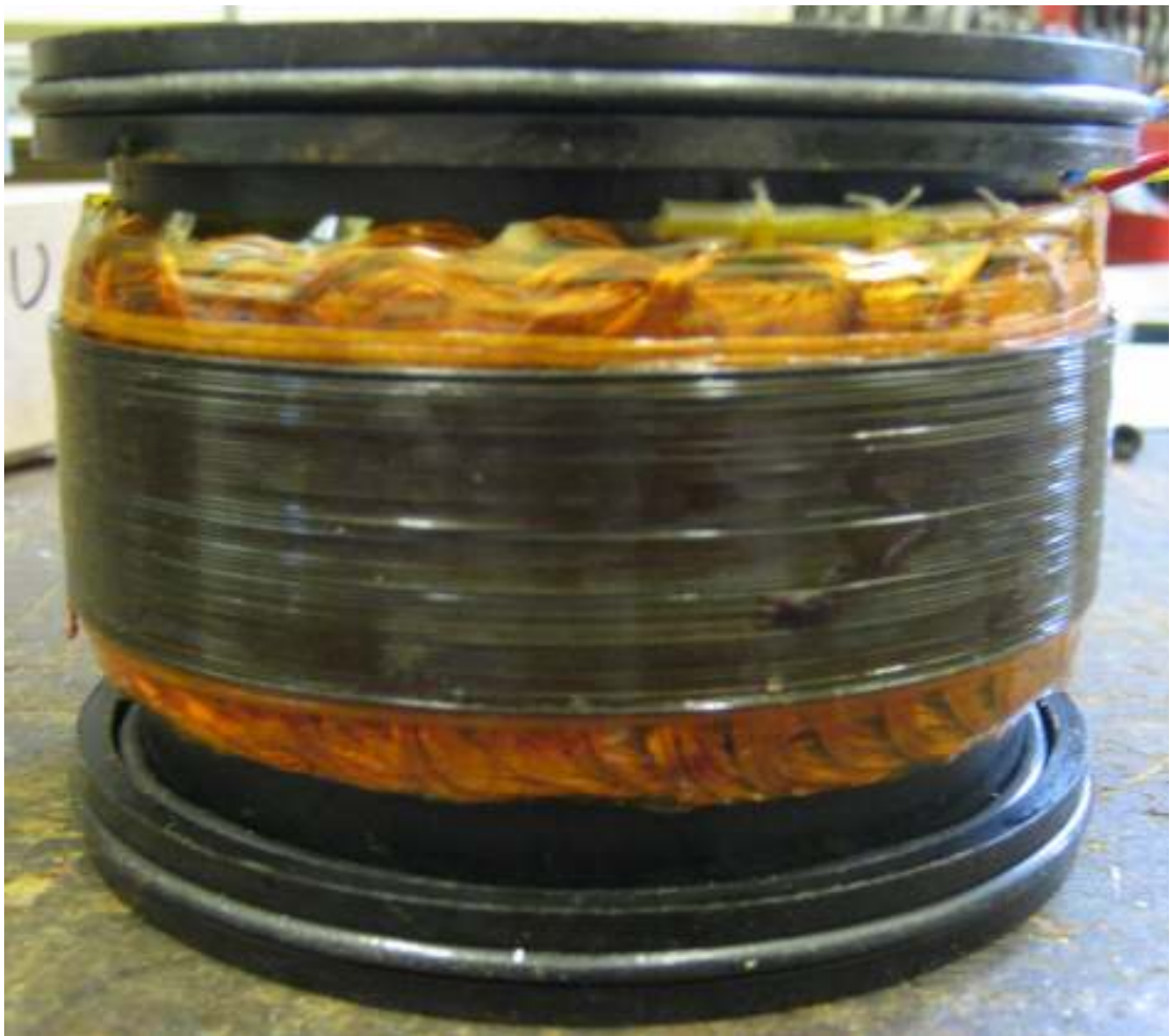
Figure 37: Completed stator-winding assembly
