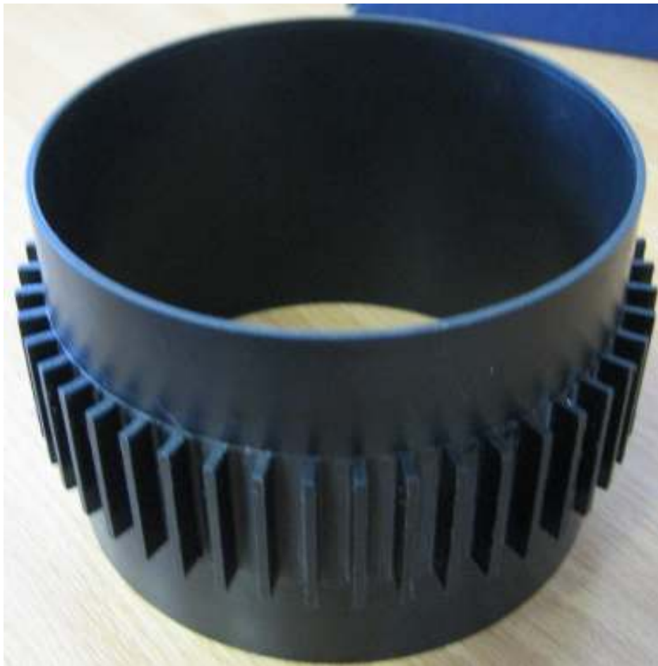
Figure 33: Picture of the former for winding coils
