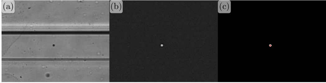
Figure S5: Sequences showing the image analysis used to estimate the wall repulsion. (a) Original unmodified frame. (b) Frame inverted and background subtracted. (c) Binarisation and noise reduction filters. The red dot marks the position assigned in the frame by the software. The example frame corresponds to 3 \mu\text{m} carboxylate particles in a 1.7 \text{ mS/m} KCl medium with 1600 Volts peak-to-peak at 50 \text{ Hz} .
