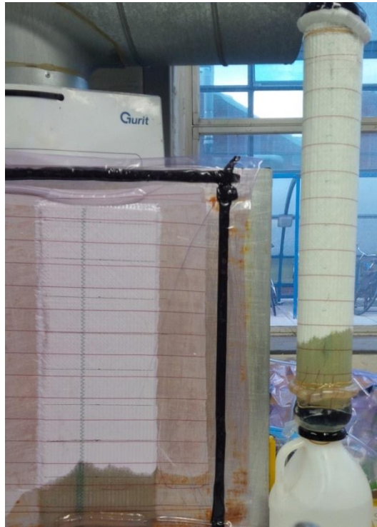
Figure 128: Vertical cylinder VARI trials against a flat rectilinear permeability experiment.
