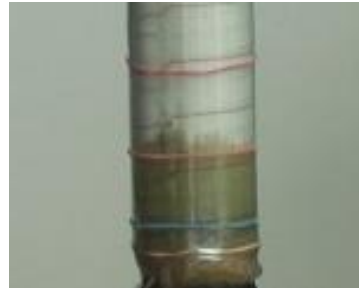
Figure 138: Resin flow front during the in-situ \mu -CT resin infusion experiment.
