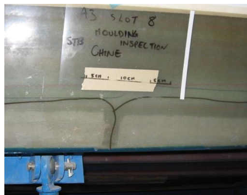
Figure 15: Void initiated fracture caused by shrinkage during cure.
