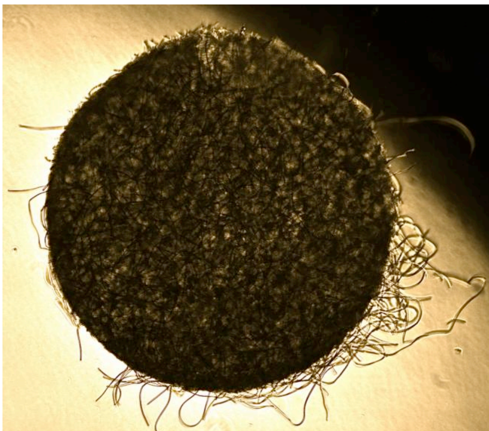
Figure 4.6: Image demonstrating that structural integrity of the 2mm diameter polymer disc was maintained even after ejection from POLARIS Mark II.
