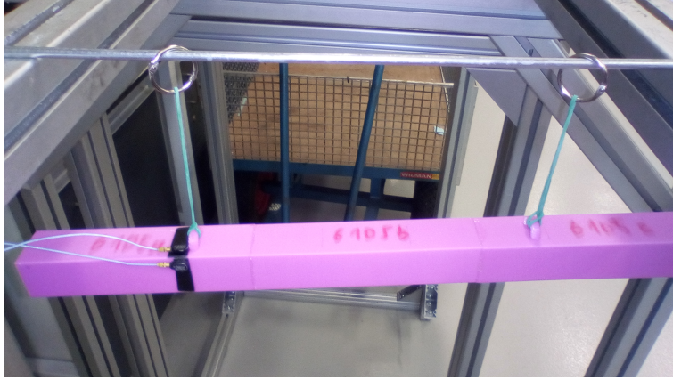
Figure 5.3: Specimens were tested in antisymmetric vibration using two accelerometers, in the transverse and vertical direction, respectively.
