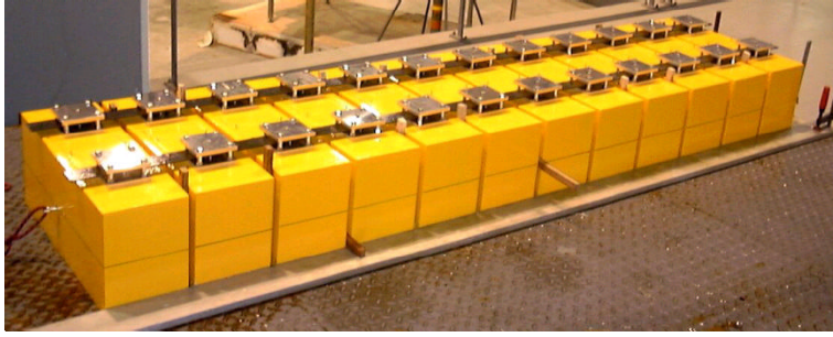
Figure 4.1: Barge consisting of 12 rectangular floaters connected by two steel backbones [27]
