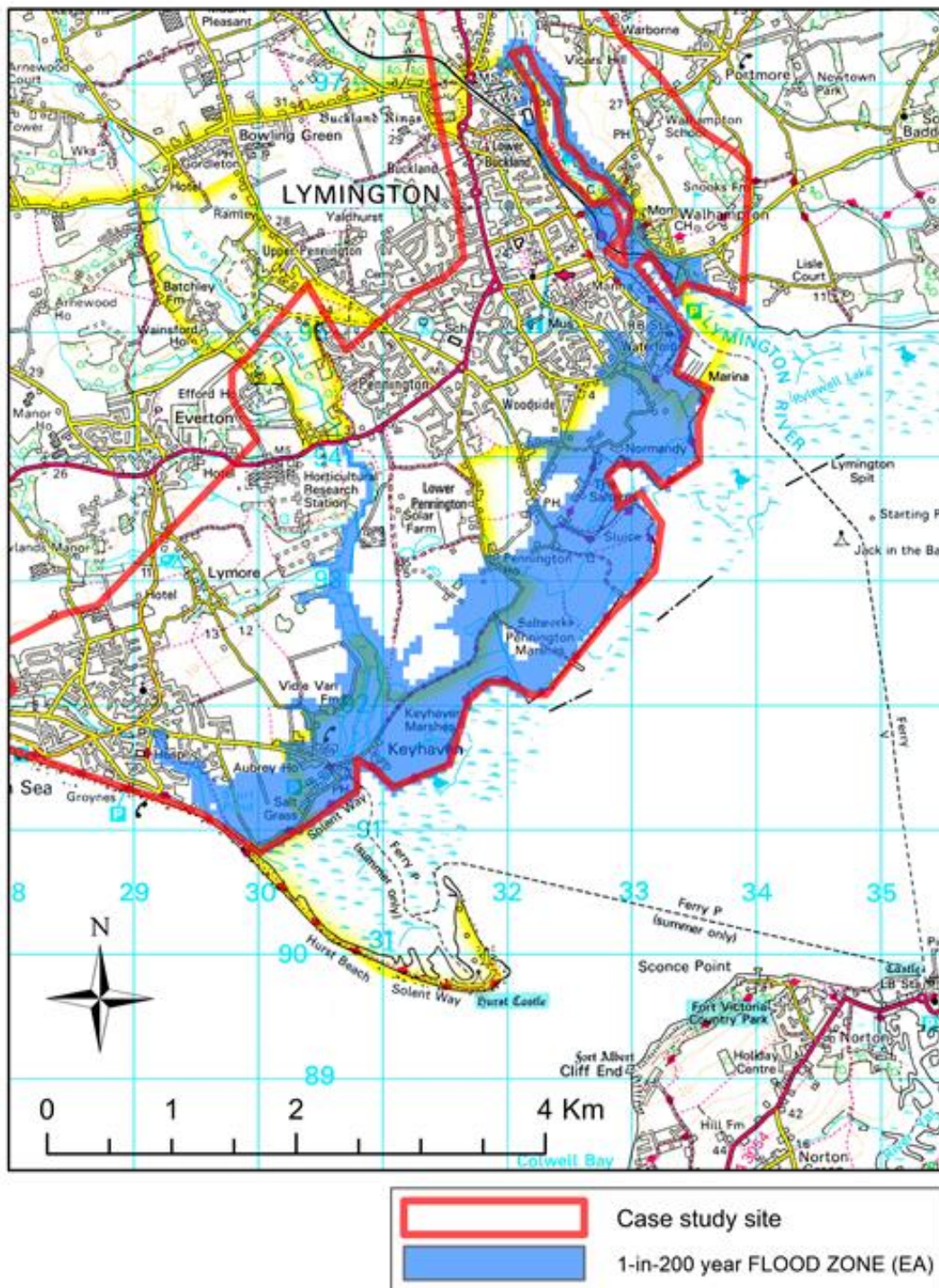
Figure 3.3 A case study area of floodplains in Keyhaven, Pennington and Lymington – Flood inundation has been simulated in hatch area.
