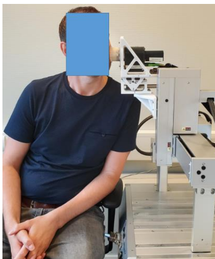
Figure 4.3 Example of a participants position when measured with the OCT system.
