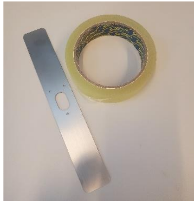
Figure 4.4 Tape stripping equipment used in session 1.
