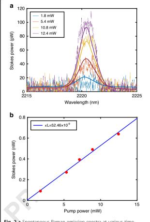
**Fig. 2 a** Spontaneous Raman emission spectra at various time-averaged pump powers, as given in the legends, for a pump wavelength of 1.99  $\mu$ m. **b** Spontaneous Stokes power as a function of coupled-in average pump power
