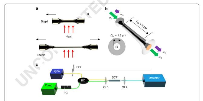
Fig. 1 a Schematic of the two-step tapering method for SCF optimization. b Schematic of tapered SCF as used for Raman scattering. c Experimental setup used for both spontaneous Raman scattering and stimulated Raman amplification measurements. OC optical chopper, BC beam combiner, PC polarization controller, OL optical lens, Detector optical spectrum analyzer/lock-in amplifier
