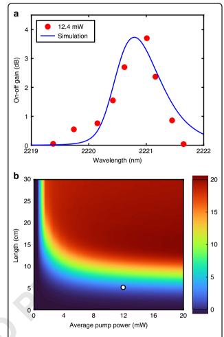
Fig. 3 a Stimulated Raman gain for a 1.99 µm pulse pump with 12.4 mW of coupled power for various signal wavelengths.
