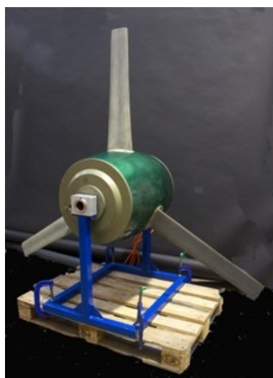
FIGURE 6.1: Picture of the tidal turbine developed at the University of Southampton.
