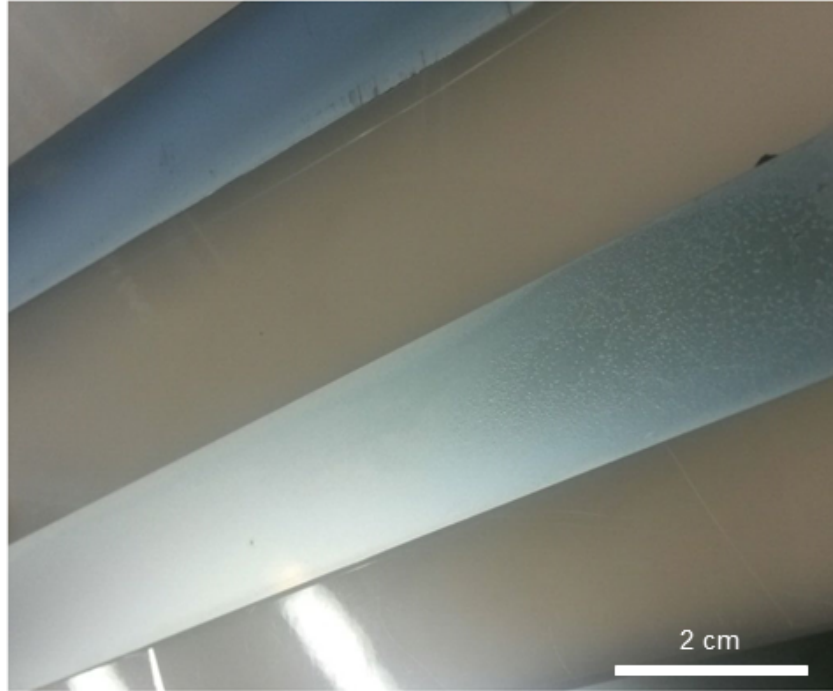
FIGURE 5.5: Two samples of MoS 2 deposited onto Si wafer substrate by chemical vapor deposition process. As we can notice on the picture, the surface is rough and reflection is very low. Therefore, the fabricated sample could not be used as a BS in the HHG process. It is an example of a bad sample which will not reflect IR light considering visually rough surface of a sample. It is important to add that MoS 2 fabrication onto some different substrates can be challenging. Sizes of samples were chosen according to the experiment design for a synchrotron source. Both samples were prepared by Katrina Morgan (University of Southampton)
