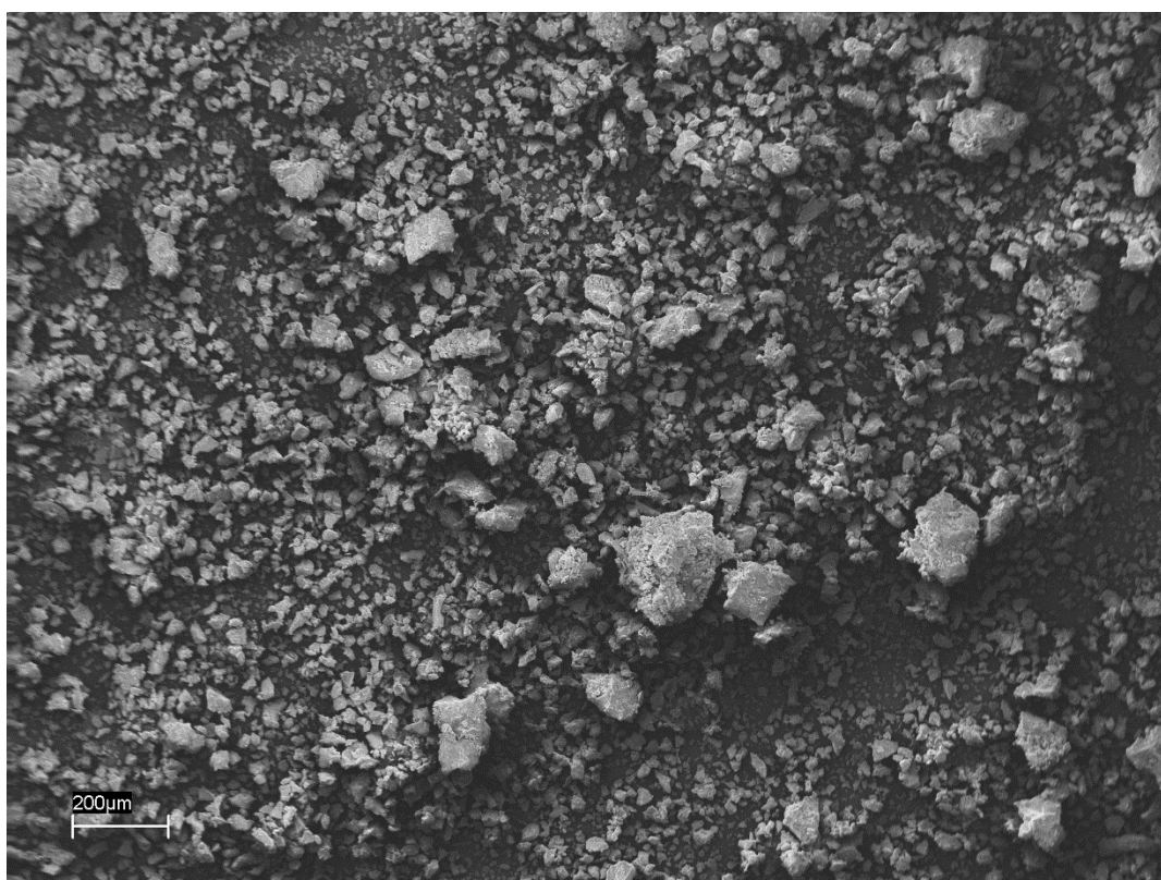
Figure 4.7: SEM image featuring a close-up of the 200 \pm 100 \mu\text{m} Clevasol test-stick showing the shape of the Clevasol particles and their distribution over a smaller space. (Magnification: 250x)
