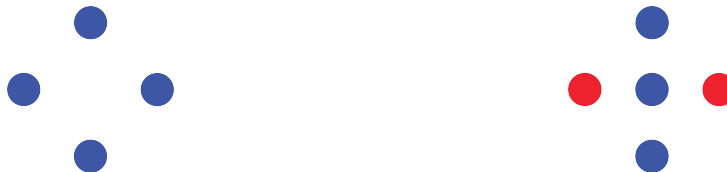
FIGURE 2.1: The class of axis-aligned rectangle classifiers has a VC dimension of four. We take the axis-aligned rectangles to classify everything with the rectangles as belonging to class “A”, and everything outside to belong to class “B”. This is because arranging four points as shown on the left-hand side, one can find a rectangle for each possible class assignment. However, adding a fifth point makes this impossible. For example, on the right-hand side configuration, there is no axis-aligned rectangle that can classify the two red points as belonging to class “A” and the three blue points to class “B”. Figure inspired by Shalev-Shwartz and Ben-David (2014) .
