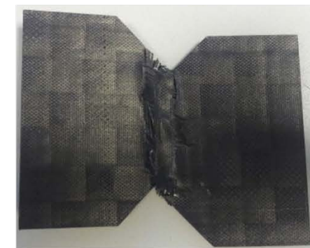
Failed shear coupon mm's - cm's (Wicaksono et al. )
