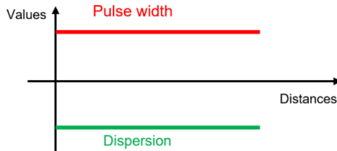
Figure 2.14: Soliton pulse evolutions with distance. This figure has been reproduced from [155], in accordance with their open access policy and terms of use.
