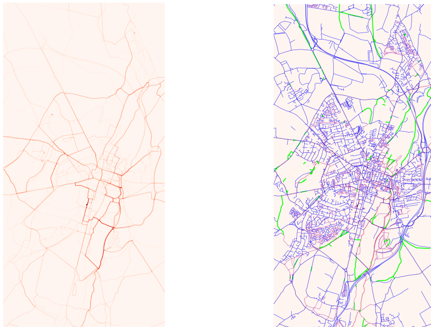
(a) LD raster - darker lines indicate greater level of use (more recorded routes). (b) LD raster overlain with MM roads (blue), paths (purple), and new paths >60m (green).
