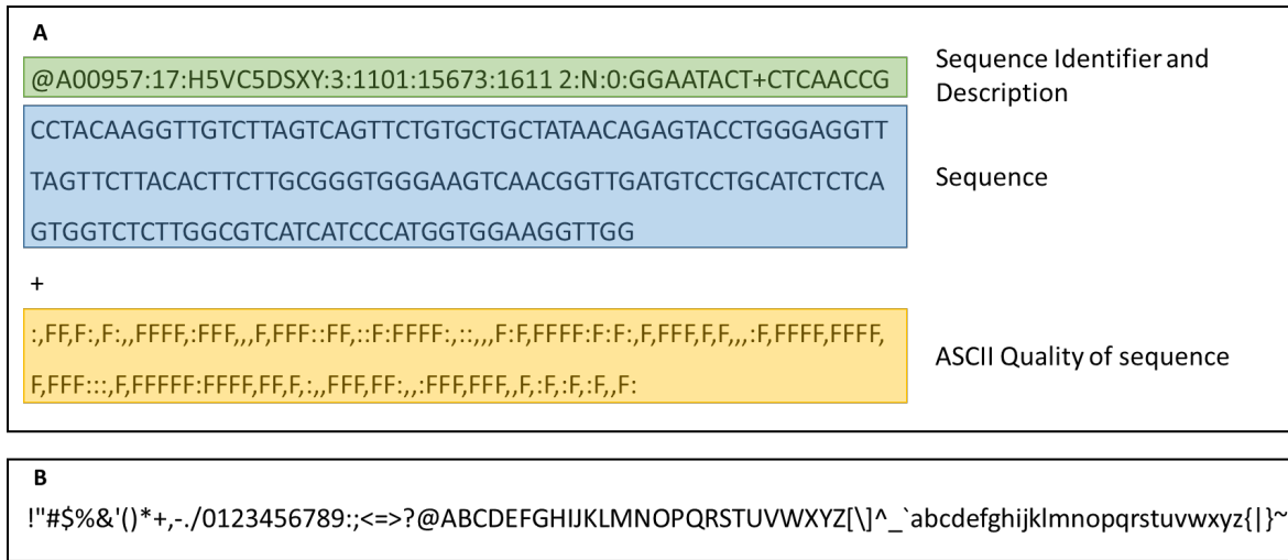
Figure 20 Fastq file format and ASCII quality. (A) Example of the fastq information format for one read. Sequence identifier and description provides information including the instrument name and run number, lane number, and if the read passed or not. (B) Lists the sequence of ASCII quality characters, with quality increasing from left to right.
