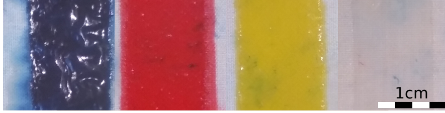
FIGURE 3.6: Four areas of interface from left to right: blue, red, yellow and clear. The blue area is much less even than the others. Uncured blue interface has bled out into the surrounding fabric.
