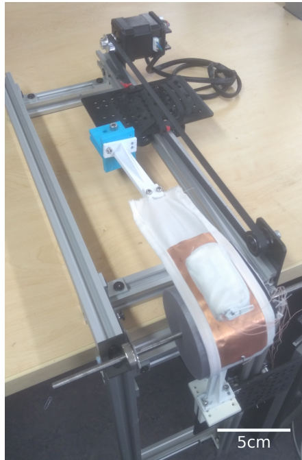
FIGURE 6.7: Test device mounted on the bespoke bending rig [18]. The real time connection between the copper sheet and each pin of the device was tested as it was pulled back and forth over the grey cylindrical axle.
