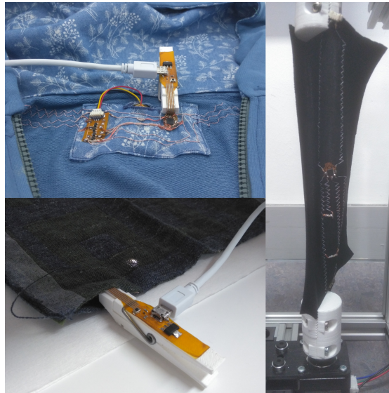
FIGURE A.3: Microcontroller circuit integrated into the collar of a garment (top left), a stretchable knitted fabric (right) and a custom woven textile (bottom left).
