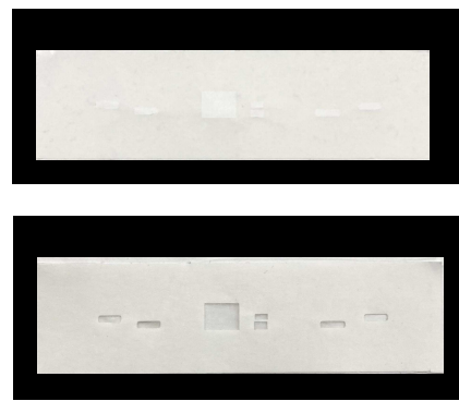
Figure 4.53 (a) Graphtec Cutting Plotter CE600-40 (b) cut samples of adhesives – NLP 11051 (top) and acrylic adhesive (bottom) (c) cut samples of Zitex G - 104 (top) and PTFE Fibre glass fabric (bottom)
