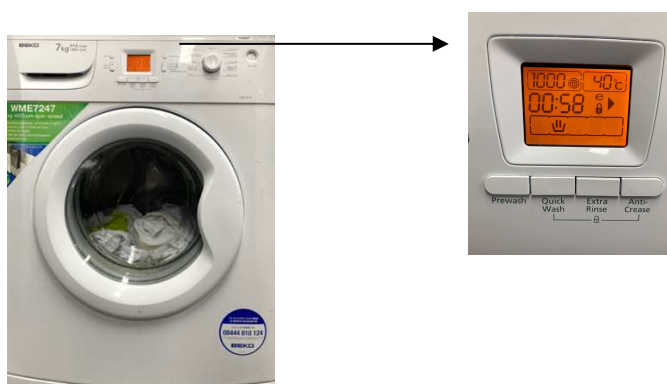
Figure 6.11 Washing machine WME7247 Beko with 58min wash cycle at 40°C, 1000 rpm and 15min spin for all the filaments
