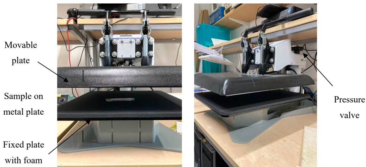
Figure 4.54 Heat press used for bonding NLP 11051 and Zitex G - 104
