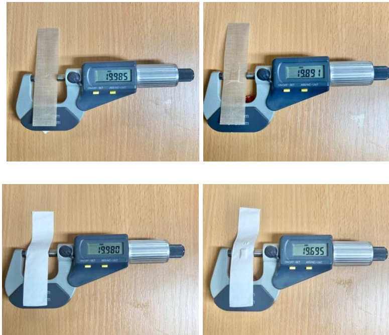
Figure 4.64 Width of the sample strip of (a) PTFE Fibre glass fabric before moulding (b) PTFE Fibre glass fabric after moulding (c) Zitex G - 104 before moulding and (d) Zitex G - 104 after moulding
