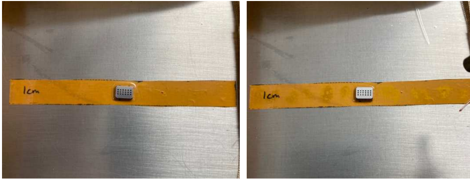
Figure 4.45 (a) vacuum formed using PU forms bubble around the chip due to straight sides (not angled) (b) reduced bubble size due to usage of heat gun and applying vacuum again
