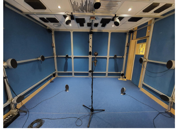
Figure 2: Room, microphone array and loudspeaker array used for the dataset generation.
