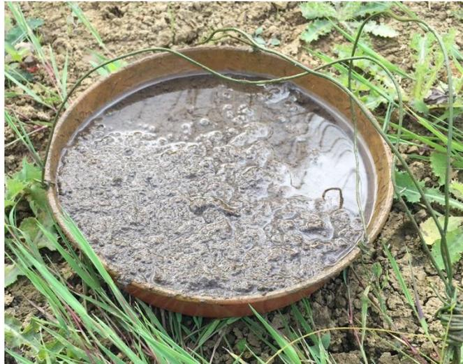
Figure 6.8: Siltation trap filled with on-line pond sediment after being deployed for circa one month.
