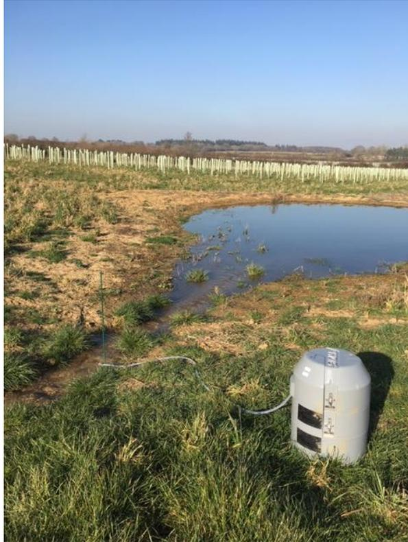
Figure 6.7: Automatic water sampler at the inlet of an on-line pond.
