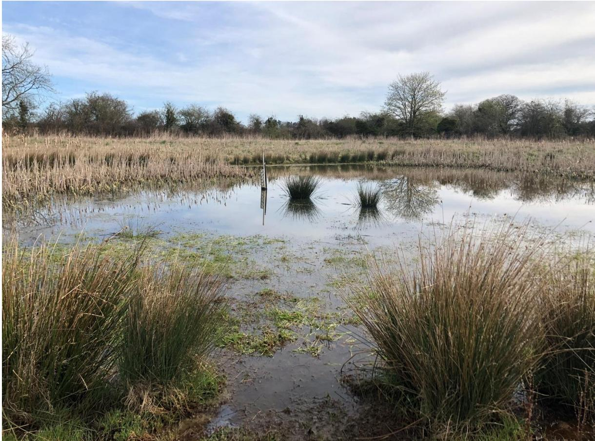
Figure 6.6: Example bund monitoring site (P3), showing stilling well containing Rugged TROLL 100 pressure sensor, mounted to wooden stake and RTK-GNSS surveyed stage board in deepest part of bund.
