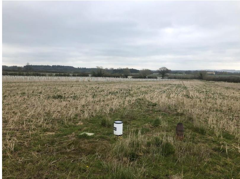
Figure 6.4: Tears of Bruern Casella tipping bucket rain gauge (left, white) and storage rain gauge (right, brass).
