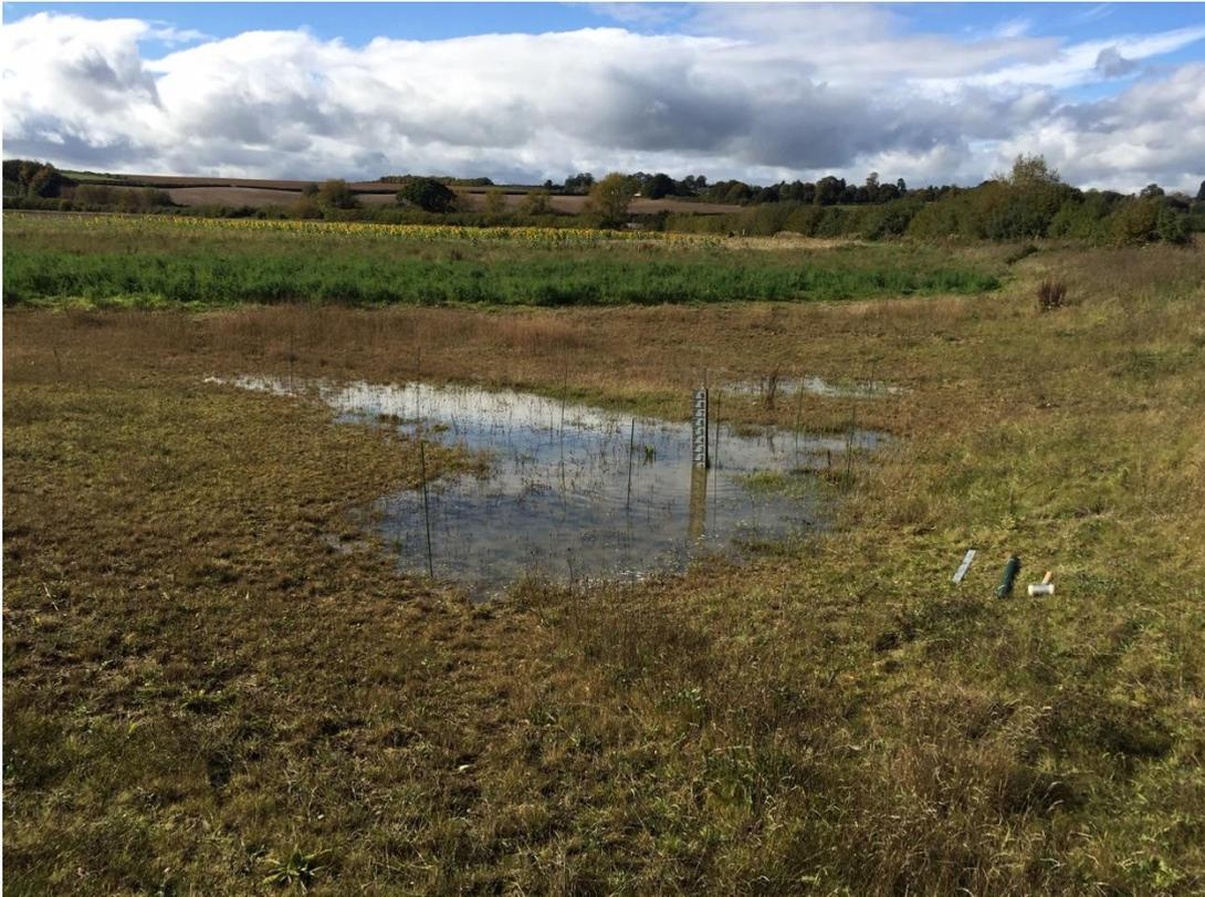
Figure 6.9: Erosion pins following installation in P6.
