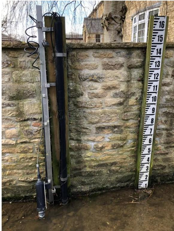
Figure 6.5: Example site set up at The Heath (TH). Showing the stage board surveyed at the right of the photo, the black stilling well mounted to the wooden board and housing the TROLL pressure sensor, and the DTS-12 turbidity sensor to the left of the stilling well.
