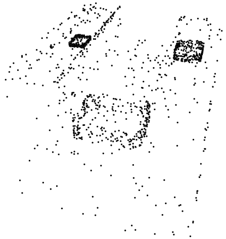
Figure 11: An example of a geometry from the Zhang machining features dataset represented as a point cloud.
