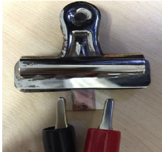
Figure 4.16. DSSC device is connected to the controller by using crocodile clips.
