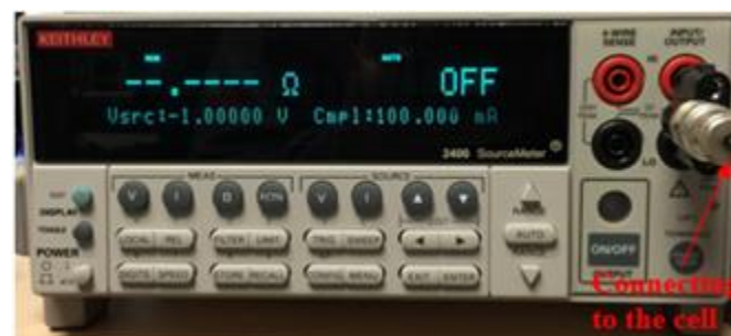
Figure 4.15. The controller of the device. This controller is connected to the cell and records the output current and voltage of the device.
