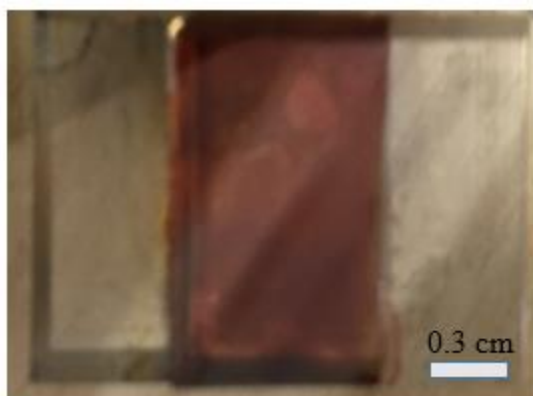
Figure 4.13. The final device of a standard DSSC, the working electrode and counter electrode assemble together.
