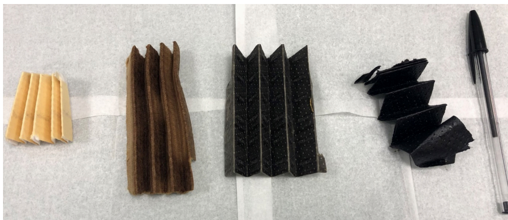
Figure 1. Examples of some of the different fuel filters analyzed, from lightly soiled on the left to heavily soiled on the right. Pen for size reference.
