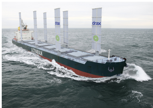
FIGURE 1.2: FastRig wing-sails developed by Smart Green Shipping ( Shipping 2023 )
