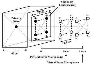
Fig. 4. Experiment setup.
