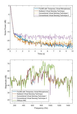
Fig. 5. The primary noise ranges from 500 Hz to 1100 Hz.
