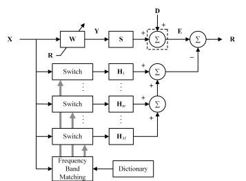
**Fig. 3**. Proposed control stage of the selective virtual sensing technique.
