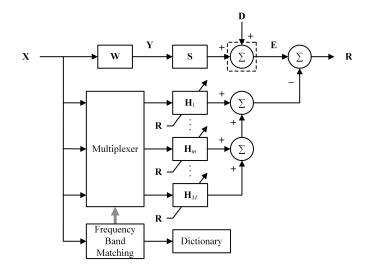
**Fig. 2**. Proposed training stage of the selective virtual sensing technique.
