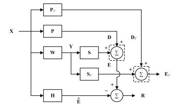
**Fig. 1**. Block diagram of the multi-channel virtual sensing technique in the frequency domain, where all notations of  $(\omega)$  have been abbreviated.
