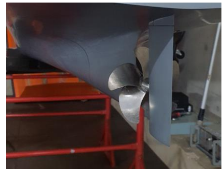
Figure 4 View from aft showing Titanium alloy propeller and all-movable rudder- gap clearance is ~ 1 mm
