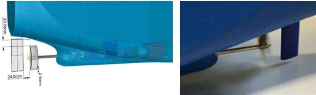
Fig. 6 – General arrangement and photo of the rudder and propeller clearance
