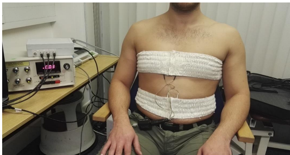
Figure 4-1: Demonstration of allocation of the RIP elastic bands around the ribcage and the abdomen
