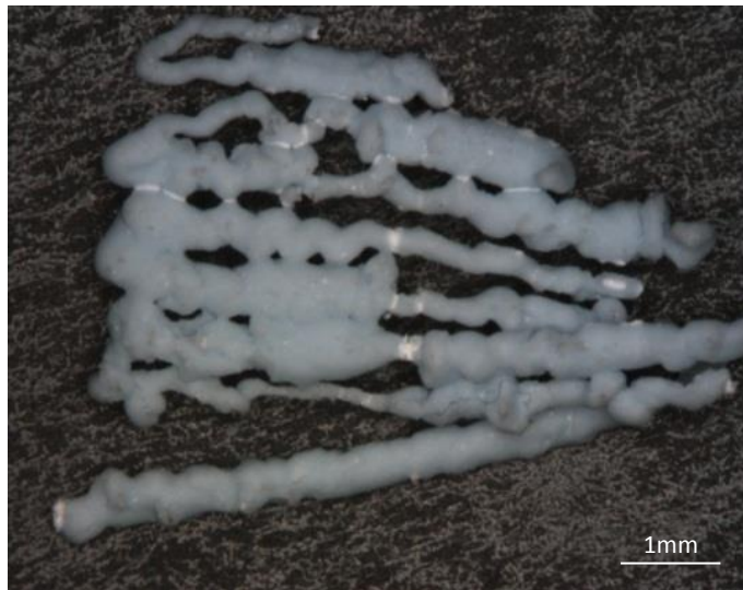
Figure A 8 Non-uniform extruded PLA/HA filaments (HA 20 vol.%)- dioxin solvent
