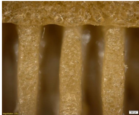
Figure 5.4 The 3D printed PEEK scaffold using filament-based extrusion system with entrapped bubbles due to polymer degradation
