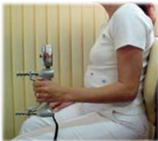
Figure 4: Position recommended for the use of the Jamar dynamometer
