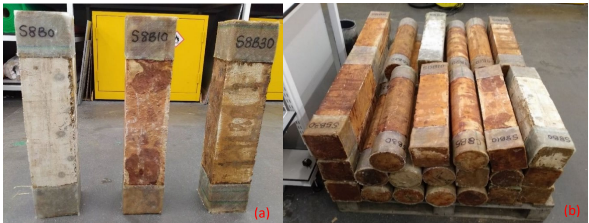
Figure 3.15. Wet layup of RC Columns (a) Individual columns (b) Completed samples before testing
