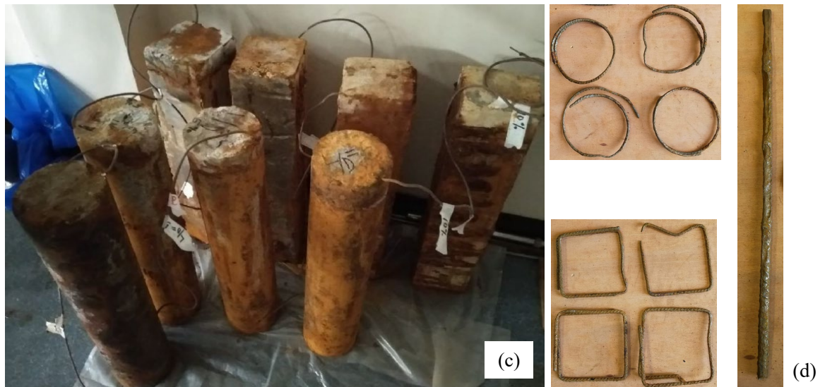
Figure 3.14. Accelerated corrosion procedure; (a) Schematic setup drawing, (b) laboratory setup, (c) corroded columns, and (d) corroded rebars after cleaning
