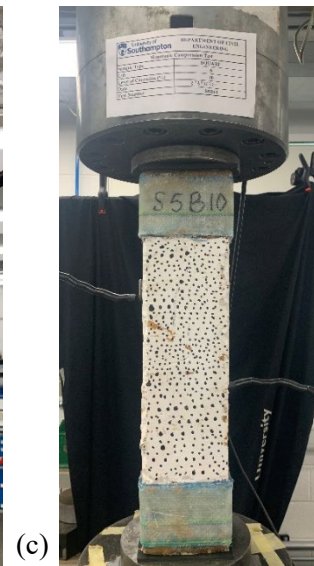
Figure 3.16: Experimental test setup (a) laboratory setup; (b) schematic of the LVDT connection; (c) Image of the LVDT connections to the R.C. samples and (d) R.C. sample with speckles for DIC
