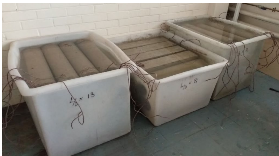
Figure 3.10: Curing the Square and Circular RC samples by complete immersion in water
