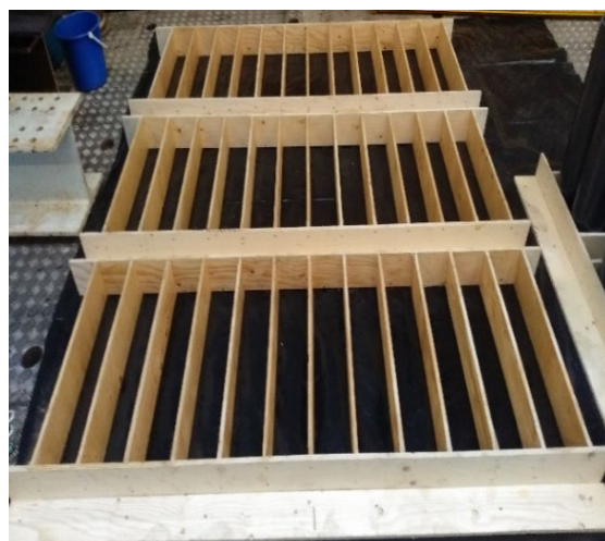
Figure 3.7: Arrangement of formworks for casting square columns - 125mm \times 125mm and 600mm long (a) Schematic drawing and (b) laboratory setup
