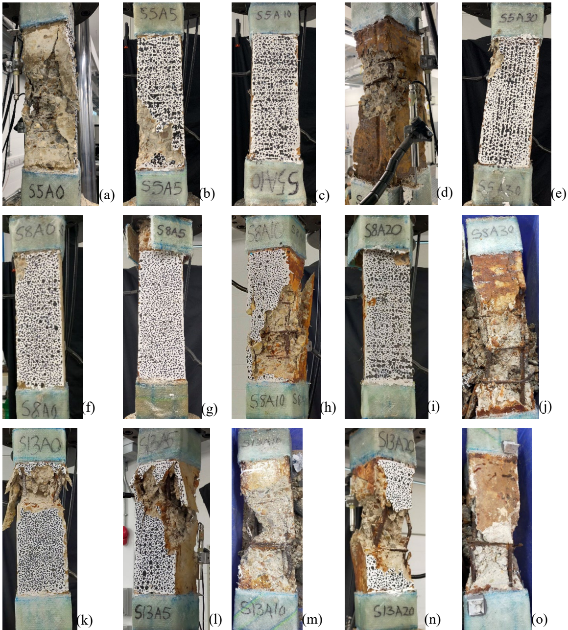
Figure 4.10: Observed failure modes of square columns with different corrosion levels and confinement ratios; L/D = 5 (a - e), L/D = 8 (f - j) and L/D = 13 (k - o)
