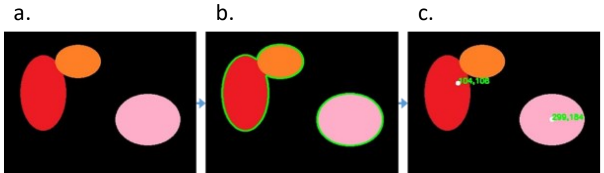
Figure 57 – in this new image example, 2 of the 3 ellipses are partially overlapping. Though to a human, the 3 ellipses are clearly distinct objects, the algorithm which has been developed so far fails to distinguish the two objects and instead treats them as one. Figure 56b shows that the contours are calculated for the combined ellipses and therefore the centroid of the combined objects is plotted on Figure 56c.
