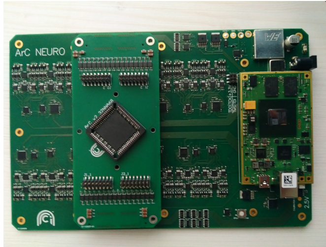
FIGURE C.1: Photograph of the block 2 ArC Neuro with FPGA module and daughterboard mounted.
