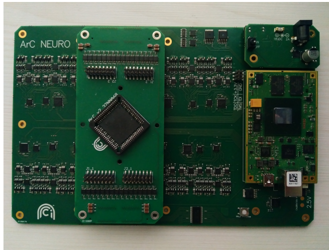
FIGURE D.1: A photograph of the block 3 ArC Neuro with FPGA module, daughter-board, and power supply module mounted.
