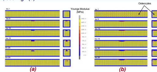
Fig 4: Longitudinal and cross-sections through the trabecular strut with (a) bone-lining cells and (b) osteocytes as mechano-sensors
