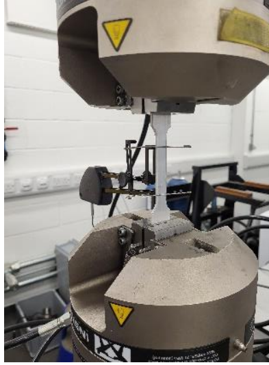
Fig. 2. Monotonic tensile test setup.
