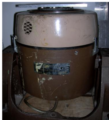
Figure 3-3 Vibrator being used to provide translational oscillation.
