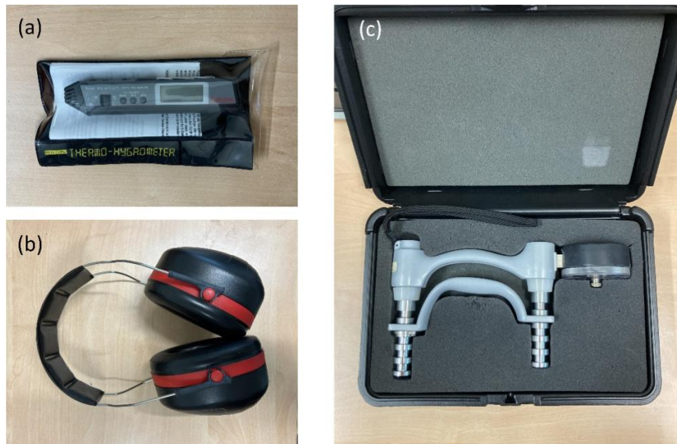
Figure 3-13 (a) A thermos-hygrometer to digitally display the room temperature and humidity. (b) Hearing protectors being worn by subjects during the test. (c) Hand dynamometer for measurement of hand grip strength.
