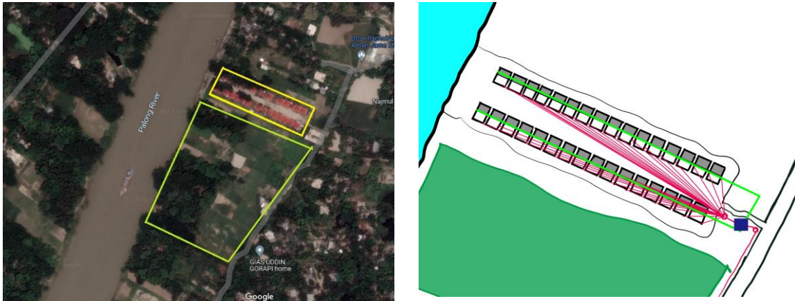
Figure 63 Interconnected Solar and main grid connection in a cluster village (Left, yellow boxed) in Bangladesh (Right, Box in the array=cluster houses, Grey= Rooftop solar, Green=Solar, Red= Main grid cable, the total solar cable length is much less than the red grid cables incurring less loss)
