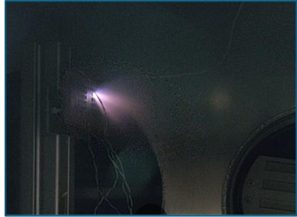
Figure 19: Image of a single pulse of the M-BMVAT with the aluminium cathode showing the plume divergence angle.
