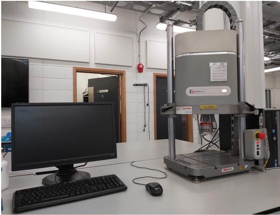
Figure 9: Photograph of the E1000 Electropuls indenter and accompanying computer.
