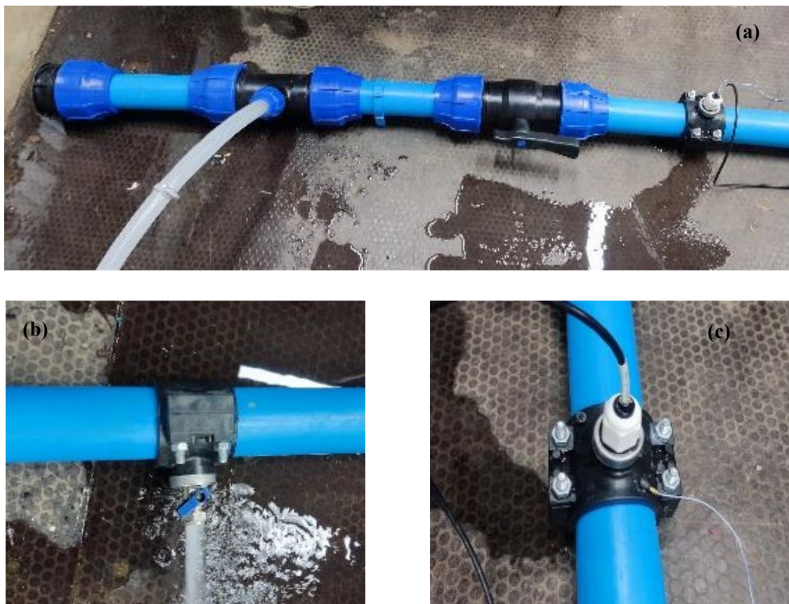
Figure 2.2: Parts of the leakage test rig: (a) Inlet section. (b) Setup for leak simulation. (c) Access points for installation of acoustic/vibration sensors.
