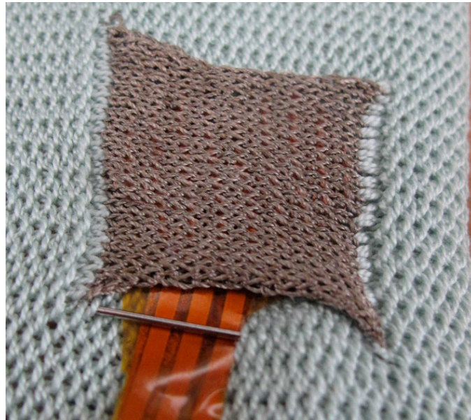
Figure 3. A knitted electrode with the op-amp circuit mounted beneath.
