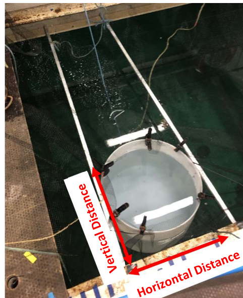
Figure 14 The experimental set up used to fulfil PhD objectives 1 and 2, showing the cylindrical tank (experimental arena, 45.0 cm height \times 55.5 cm diameter) inside a large tank (8.0 m length \times 8.0 m width \times 5.0 m depth) in relation to the water level (dotted line, 30.0 cm depth). The transducer was suspended 70 cm below the tank, and a hydrophone placed 15 cm below the water level and 20 cm away. The vertical and horizontal distance have been labelled and were used for the researcher to undertake acoustic mapping.
