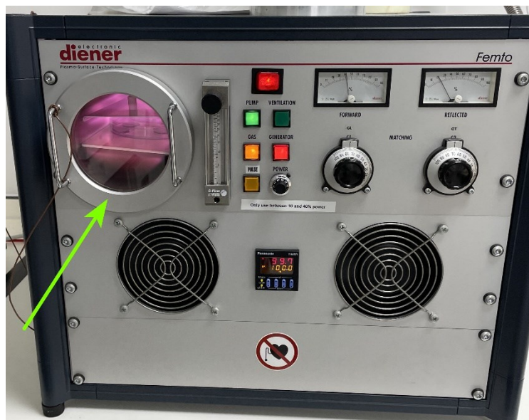
Figure E6. Glass beads underwent oxygen plasma treatment to activate the surface silanol groups, employing a plasma activation system (Diener Electronic, Ebhausen, Germany). The effectiveness of the plasma treatment was assessed by observing the behaviour of water droplets on the beads. Resistance to wetting by beads indicated successful plasma treatment (Subeshan et al. 2020).
