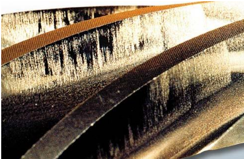
Figure 2-18 Scuffing Damage to Helical Gear Tooth [25]
