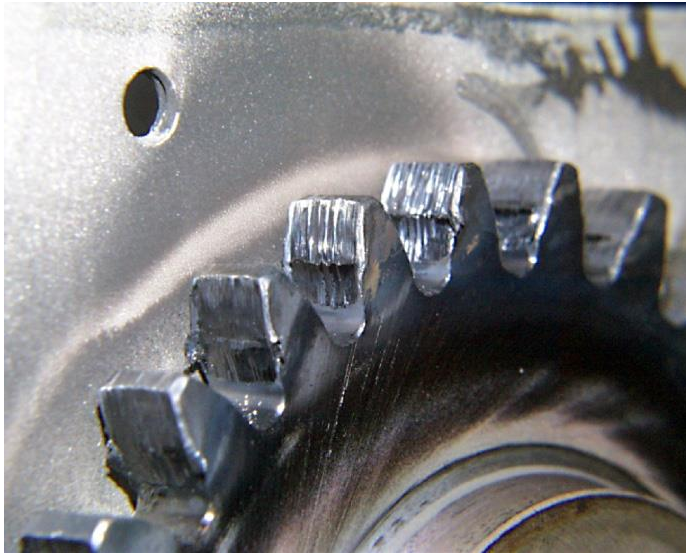
Figure 2-23 Failure of a Spur Gear Following Loss-of-Lubrication Testing [54]
