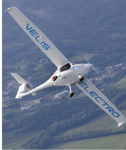
FIGURE 3.1: Pipistrel Velis Electro, the world's first EASA Type-Certified electric aircraft. Photo by [131].
