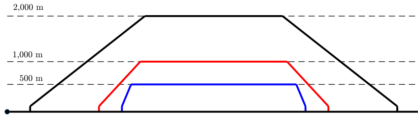
FIGURE 9.6: Vertical flight profiles possibilities. Flight altitude is determined by total distance covered.
