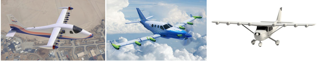
FIGURE 3.5: DEP concept renderings, from left to right: 1. NASA X-57 Maxwell, 2. Airbus EcoPulse™, 3. ISVR DEP Cessna 172 (model designed and rendered by author for illustration purposes).
