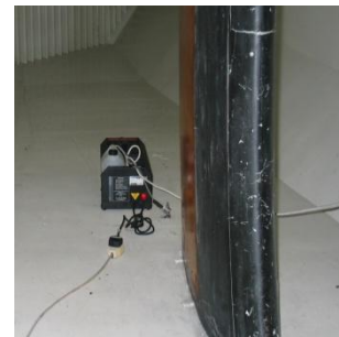
Figure 5 - The smoke machine downstream the wind tunnel.
