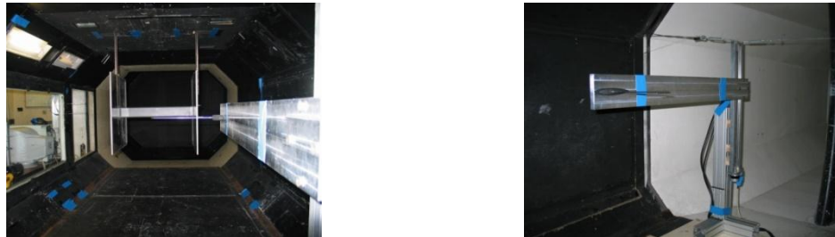
Figure 8 - The pitot-static tube downstream of the mirror (left) and the traverse system (right).
